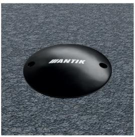
**ANTIK LoRaWAN parking sensor surface-mounted** allows citizens and municipalities to detect occupancy of specific parking lots. Sensor continuously monitors status of parking lot using sensitive geomagnetic sensor. The occupancy change is immediately transmitted to the master system. Device is easy to install by mounting it on the surface of the parking lot and fastening two screws in the dowels.
